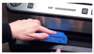
To access the upper gasket and bag sensor hinges, open the drawer and gently flip your vacuum sealer completely over with the drawer open.
