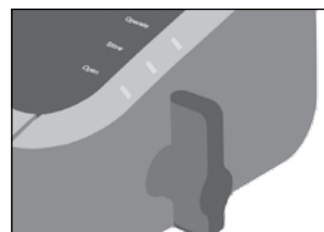
Push the latch into the center position to store.
